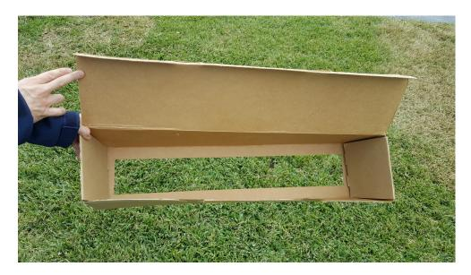
Then place the **Spray Box** along your stencil lines and start painting. This box will help you apply pressure to the stencil so that everything makes good contact with the ground and to keep you from over spraying onto your court area.
