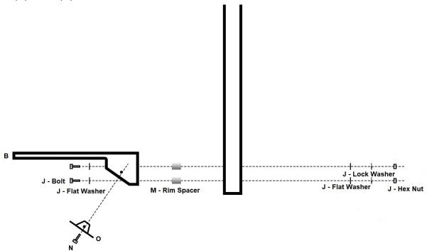
**NOTE**: Use a level to make sure rim is level side to side before tightening nuts
