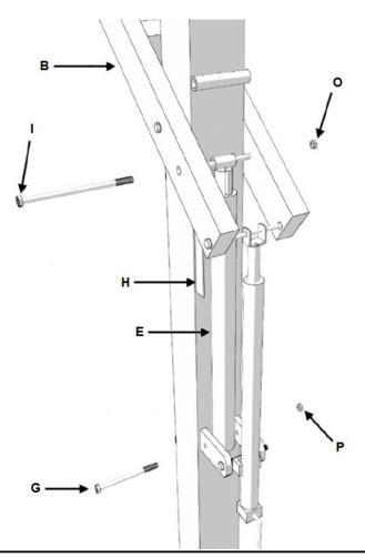
**NOTE:** Tighten the lock nuts down and then back off a 1/4 turn to allow the joint to pivot when adjusting the system up and down.
