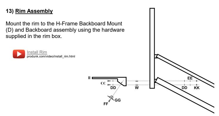
**NOTE**: Use a level to make sure rim is level side to side before tightening nuts
